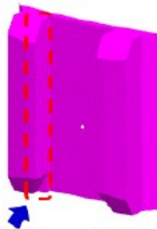
Core Support Snubber Lug
